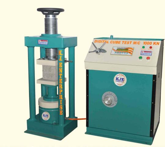
DIGITAL 1000 KN COMPRESSION TEST M/C.
