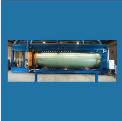
Pipe Hydro-Testing Machine (PHTM)
